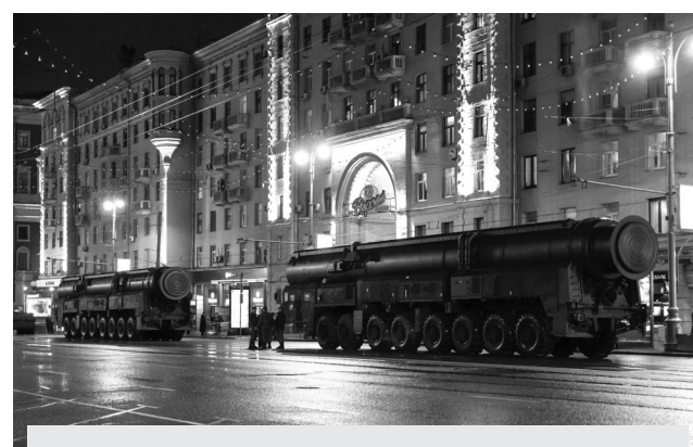
Russia's RT-2PM2 Topol-M space intercontinental ballistic missiles, cold-launched, three-stage, solid-propellant, road-mobile intercontinental ballistic missiles with thermonuclear warheads. Rehearsal for Victory Day Military Parade in Moscow, Russia. Photo courtesy of The Commons
